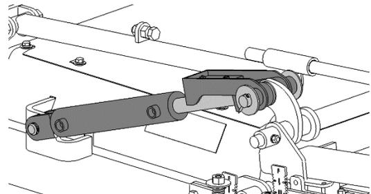
20) Connect the outer wing lift circuit to a hydraulic power source (tractor or power pack) and extend the cylinders until they align with the mounting brackets on the lift pivot bar. Connect cylinder and lift stop to lift pivot bar using pin & hardware on cylinder as shipped.
