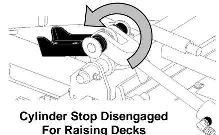
**Cylinder Stop Disengaged
