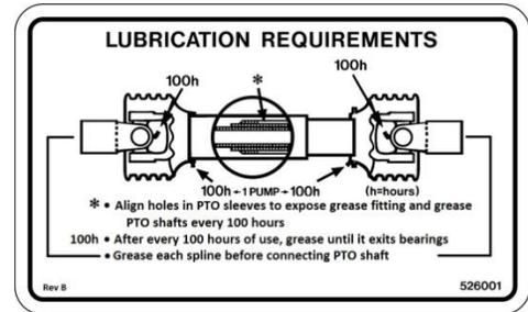
**INPUT & DECK SHAFTS – 100h / Monthly (7 / Shaft - 6 Shafts)**
