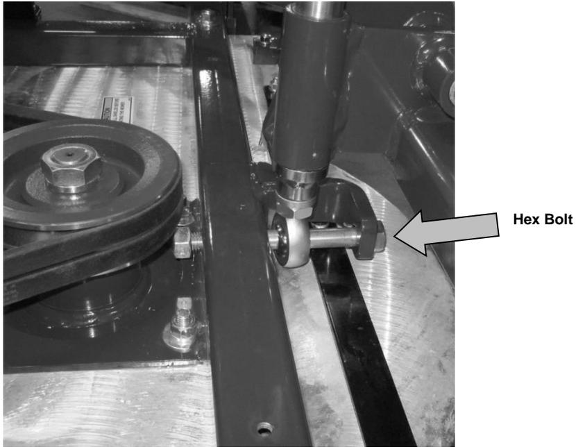
9) Remove the 5/8" x 6 hex bolt from the deck frame and install it through the lift shaft tie rod.
