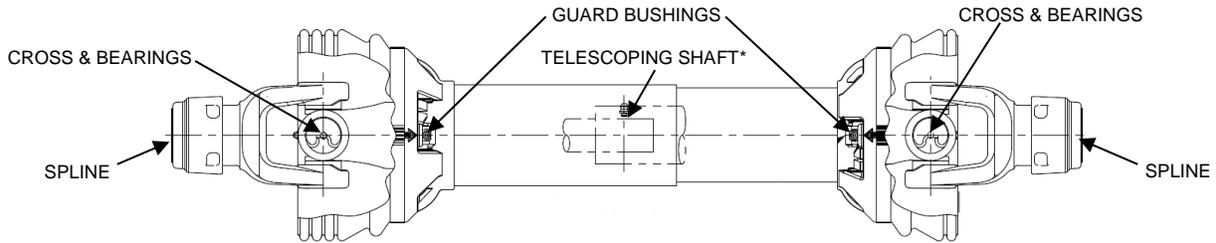
\* Inner & outer guards must be rotated to align holes for accessing telescoping shaft grease fitting.
